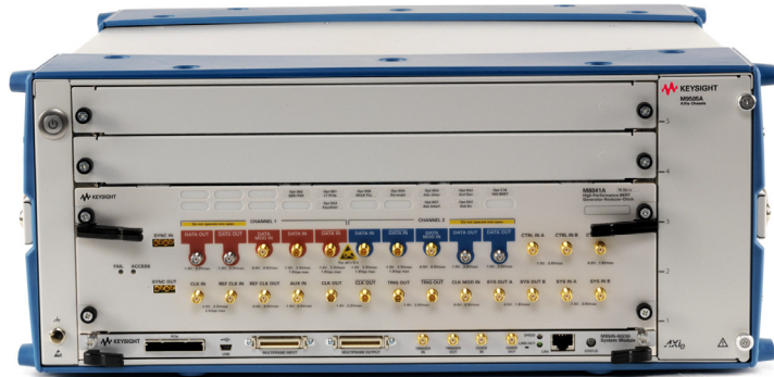
Figure 1 M8020A configuration for 16 Gb/s BERT with 1 to 2 channel
